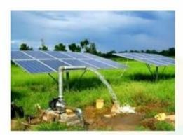
Helius Solar Water pump is an independent stand-alone system, which works from dusk to dawn and are available in different types and capacity. It offers a clean, efficient and simple alternative to fuel burning enginesand generators for domestic water, livestock watering drip irrigation, remote houses and where water is needed but no AC power is avaiable. They are most effective during dry and sunny seasons. They require no fuel deliveries and very little maintenance.
